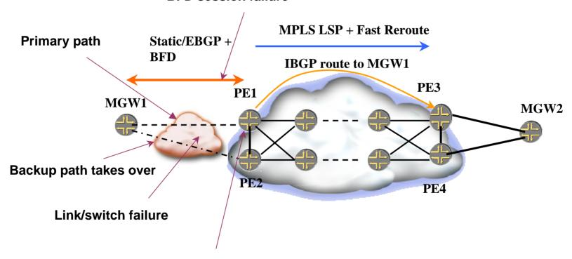
PE1 switches to a backup route through PE2 to reach MGW1
